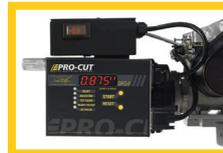
**Step 3:** Computer compensates for lateral run-out
