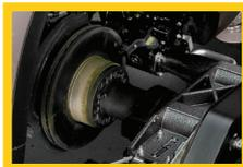
**Step 2:** Attach the lathe to the adaptor
