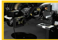
**Step 4:** The PFM X9 DRO resurfaces both faces of the disc simultaneously
