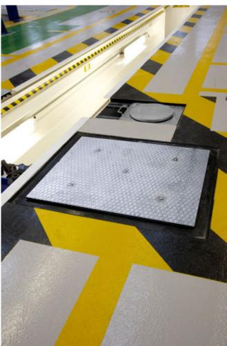
The DE/7353 hydraulic play detector is designed for testing of Heavy Goods Vehicles (HGV) and Public Service Vehicles (PSV) in accordance with the UK statutory test.
