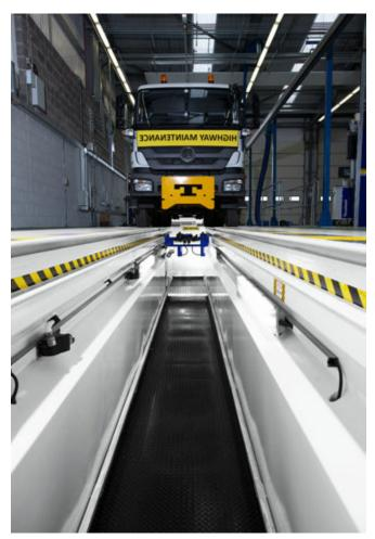
Today, commercial vehicles are still commonly serviced with pits rather than on lifts. Firstly, it allows for quicker throughput, which means the vehicles can be serviced faster. Secondly, minimal maintenance is required for pits, making them a cost-effective option. Finally, pits marked with CE 1090 offer improved health and safety measures.
