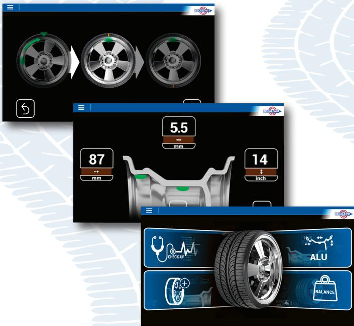
The Wave 5 series electronic Wheel Balancer comes equipped with either a 22" interactive touchscreen monitor (idea for high volume of tyre shops) or a colour 7" LCD display with integrated keyboard. The design and interface allows for high performance and accuracy when balancing most types of car, motorcycle and van wheels.
