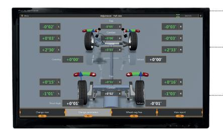
A comprehensive vehicle database covering over 40,000 vehicles is integrated into the operating program. It includes wheel alignment specifications, tyre pressure data, vehicle adjustment diagrams and images together with **3D animated videos**.
