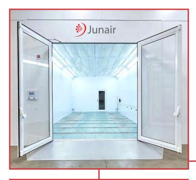
A LEVAC floor is a surface mounted design requiring no building excavation. Height from the building floor to the spray booth floor is only 180mm and only a small unobtrusive ramp is required to access the cabin, making it easy to load and unload products. Removing the excavation element significantly reduces installation time /costs and the disruption associated with builder's work.
