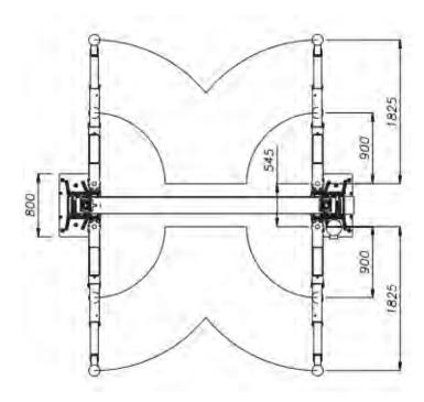
Lifting Capacity: 5500Kg
