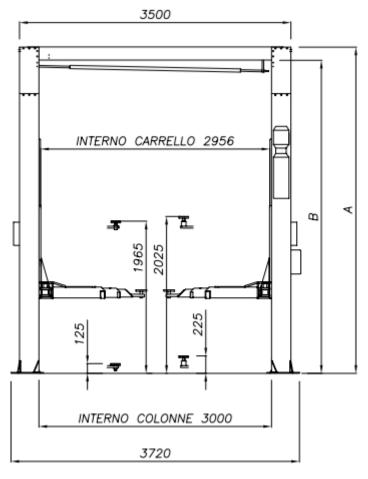
SF/9195/A =Standard Height SF/9196/A/LH = Low Height A =5100mm A =4200mm B= 4930mm B= 4030mm
