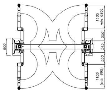
Lifting Capacity: 5500Kg
